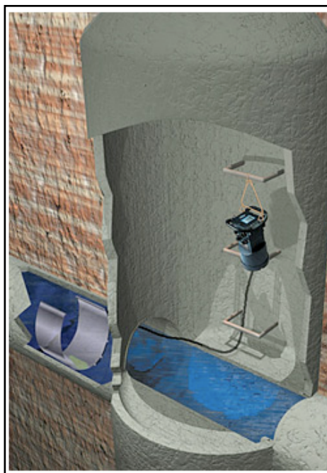
Figure 5: Basic configuration of the flow sensor. Logger is mounted to the manhole ladder. Flow sensor is mounted using a spring ring. This study uses three sensors in three pipes. (HACH 2011)
