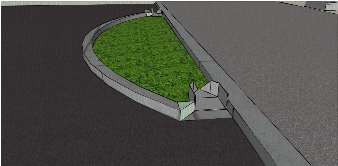
Conceptual Green Infrastructure Design: Example of flume orientation and design for the bump-outs and right-of-way bioswales (in preparation).
