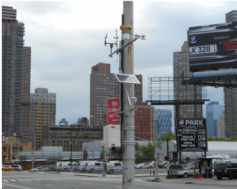
Climate Station: Example of Climate Station Mounted on a street pole adjacent to the Jacob Javits Center in Manhattan.
