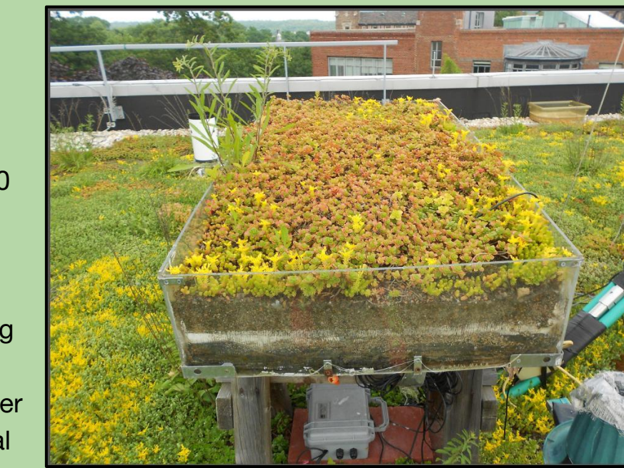
Drainage from the lysimeter is measured using a tipping bucket rain gage
